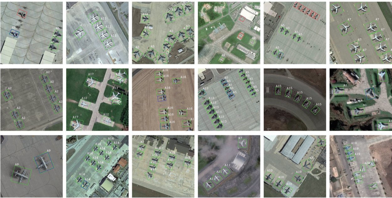
图3 有向框飞机目标识别结果可视化(绿框代表正确识别结果,红框代表漏检,蓝框代表虚警) Fig. 3 The visualization of aircraft recognition results with oriented boxes (The green boxes represent true positives , red boxes represent false negatives and blue boxes represent false positives )
