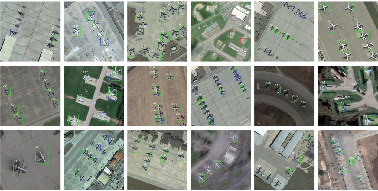
图2 水平框飞机目标识别结果可视化(绿框代表正确识别结果,红框代表漏检,蓝框代表虚警) Fig. 2 The visualization of aircraft recognition results with horizontal boxes (The green boxes represent true positives , red boxes represent false negatives and blue boxes represent false positives )
